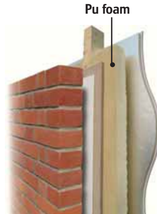
Timber frame wall
